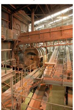
In the first step of the superten manufacturing process, sulphuric acid (usually diluted to 70% concentration) is added to a mixer, along with the phosphate rock. Paddles in the mixer help ensure the material is thoroughly mixed, a process that takes less than one minute.
