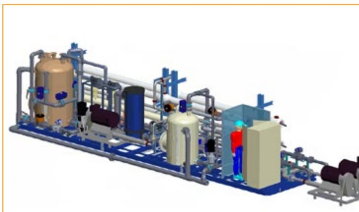
**Hiprode**, a totally new design in RO seawater desalination units. It allows optimum use of the greater permeability of the new membranes available on the market, thereby improving efficiency and reducing the size of the facility and its cost. The prototype tests conducted on this new configuration in a desalination plant operated by Veolia in Gibraltar were completed with success at the end of 2014, allowing the integration of this technological improvement in VWT’s offering.
